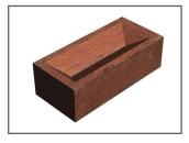
silicate are also used. They are categorised by use – i.e. facing, common and engineering bricks – which relate to their strength, durability and frost resistance. The outer leaf of a typical cavity wall is constructed from facing bricks which, depending on the required finish and budget, can be either handmade, stock or wirecut, each of which describes the manufacturing process used and will determine the external appearance.
