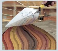
Mortars can be pigmented to highlight, enhance or tone in with the masonry used. The colour of the mortar joint can totally change the appearance of the finished masonry and a comprehensive range of colours and shades are available from suppliers of factoryproduced mortars.
